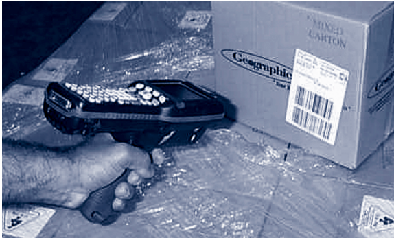
Figure 11: Use of hand-held scanner to read GTIN code at Coles-Myer (K-Mart) DC
